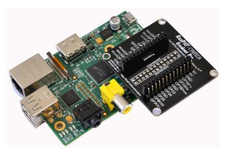
Solder the main 26-way female header underneath first, then the inner (female) and outer (male) headers on top, according to your preference. Ensure the board is attached to the Raspberry Pi<sup>®</sup> as shown above. (Raspberry Pi<sup>®</sup> not included)
