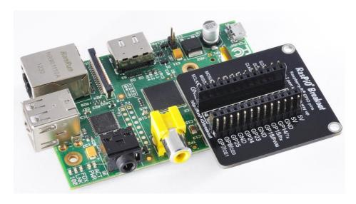
Decide whether to assemble as Rev 1 or Rev 2. Solder the main 26-way female header underneath first, then the inner (female) and outer (male) headers on top, according to your preference. Ensure the board is attached to the Raspberry Pi® as shown above. (Raspberry Pi® not included)
